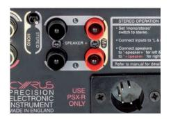
With benefits for sound quality, it is possible to connect an optional PSX-R network component, and the X Power can also be operated as a mono set.
