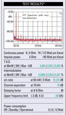
LABORATORY COMMENTS: Respectable output performance, certainly sufficient for most applications with substantial spare capacity and top-quality values in all important categories such as extremely low distortion and low noise.
